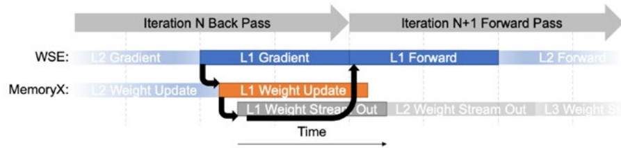
Figure 23. Pipelining of weight and gradient communication between the MemoryX service and the WSE-2.
